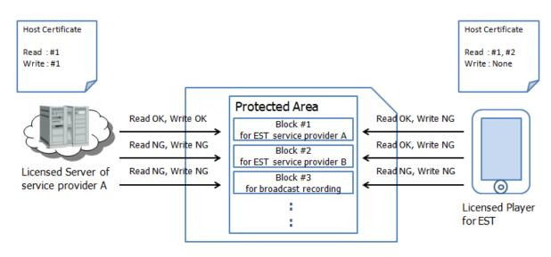
Figure 3-3 Access control of the Protected Area
