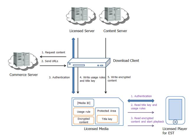
Figure 3-1 Components and flow in the case of EST
