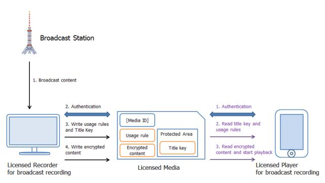
Figure 3-2 Components and flow in the case of broadcast recording
